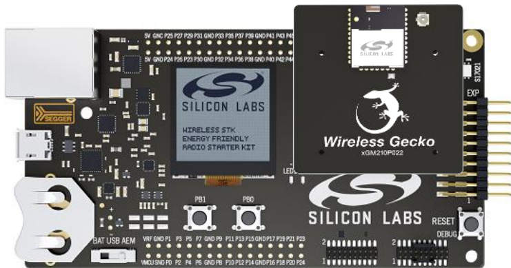
Wireless Starter Kit (WSTK) main board
